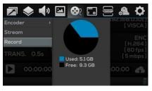
used capacity and available capacity of the USB flash drive. Click the REC button to start recording. The file name of the recorded file will appear below the pie chart, and the REC light will flash. Press REC again to stop recording.
